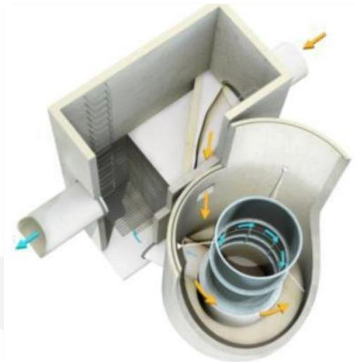
Figure 24 – Schéma de principe CycloneSep
